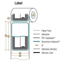
\*Antenna Thickness: (0.0003 in) I \*\*PET Thickness: 0,05 mm (0.002 in) I Yield, Joint: 297%, ≤2p/roll
